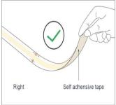
If the led strip needs to be torn up,please make sure that the self adhensive tape is torn with the led strip,otherwise the led strip will be damaged.
